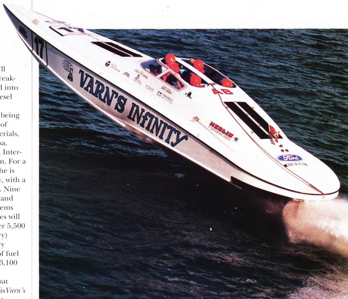
Driven by three triple turbo diesels, Varn's Infinity can reach a top speed of 96 mph.
