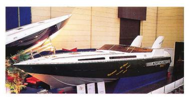
hese two aluminium hulled craft are very special. Both prototypes, they are test beds for a new generation of gas turbine propelled sports cruisers and they aroused a great deal of attention at Dusseldorf. It is easy to see the attraction of gas turbines for sports cruisers, they are compact and light weight, smooth running, and they offer tremendous power outputs from a small package. However they are expensive and potential owners may be put off by the cost.
