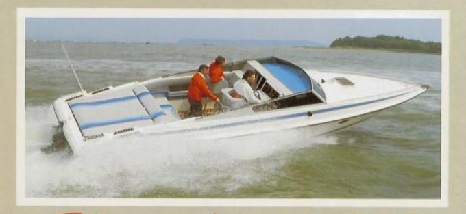
The well laid out cockpit area provides good all-round vision when seated in the padded helmsman and pilot seats. To minimise the glare from the water most boats are fitted with a darkened wrap around windscreen. There is additional seating for visitors in the cockpit, with a further area for sunning or relaxing after swimming on the rear cushloned sun-deck.
