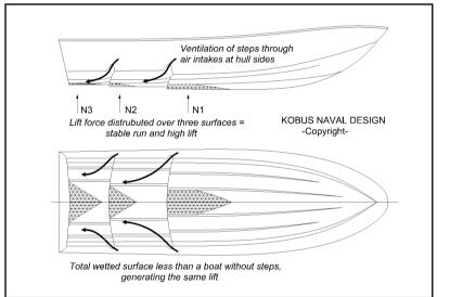
added speed from a stepped bottom is due to a layer of bubbles that undoubtedly reduce frictional drag (true to some extent), but the real saving is in minimizing the hull area in contact with the water, specifically by presenting two or three wide and short surfaces to the water instead of one long, narrow one.
